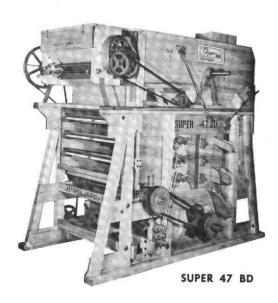
In this series B designates 3-screen construction — D designates dustless or top fans construction.
