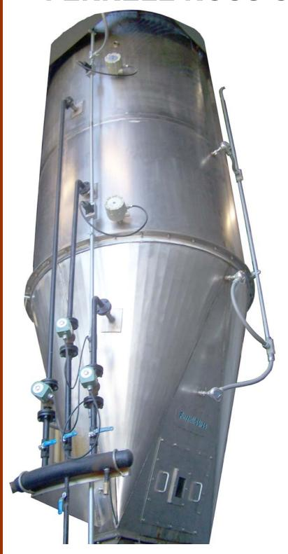
Ferrell-Ross Steam Chests are robustly constructed of 10 gauge 304 Stainless Steel. Our sharply sloped cone section ensures Mass Flow and provides first-in-first-out cooking with no rat holing, bridging, or other flow problems. Our steam chest uses exclusive rolled ring steam injection design which produces an excellent cook.
