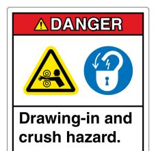
Lockout power before removing guard, cover or inspection door.
