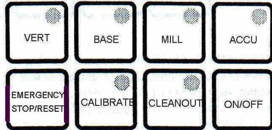
The EMERGENCY STOP/RESET button is used to clear any trouble indicator after the problem has been corrected. The emergency stop causes an immediate shutdown of the entire mill during any mode of operation. After this feature is used, the grinding chamber must be cleaned out before restarting the mill.
