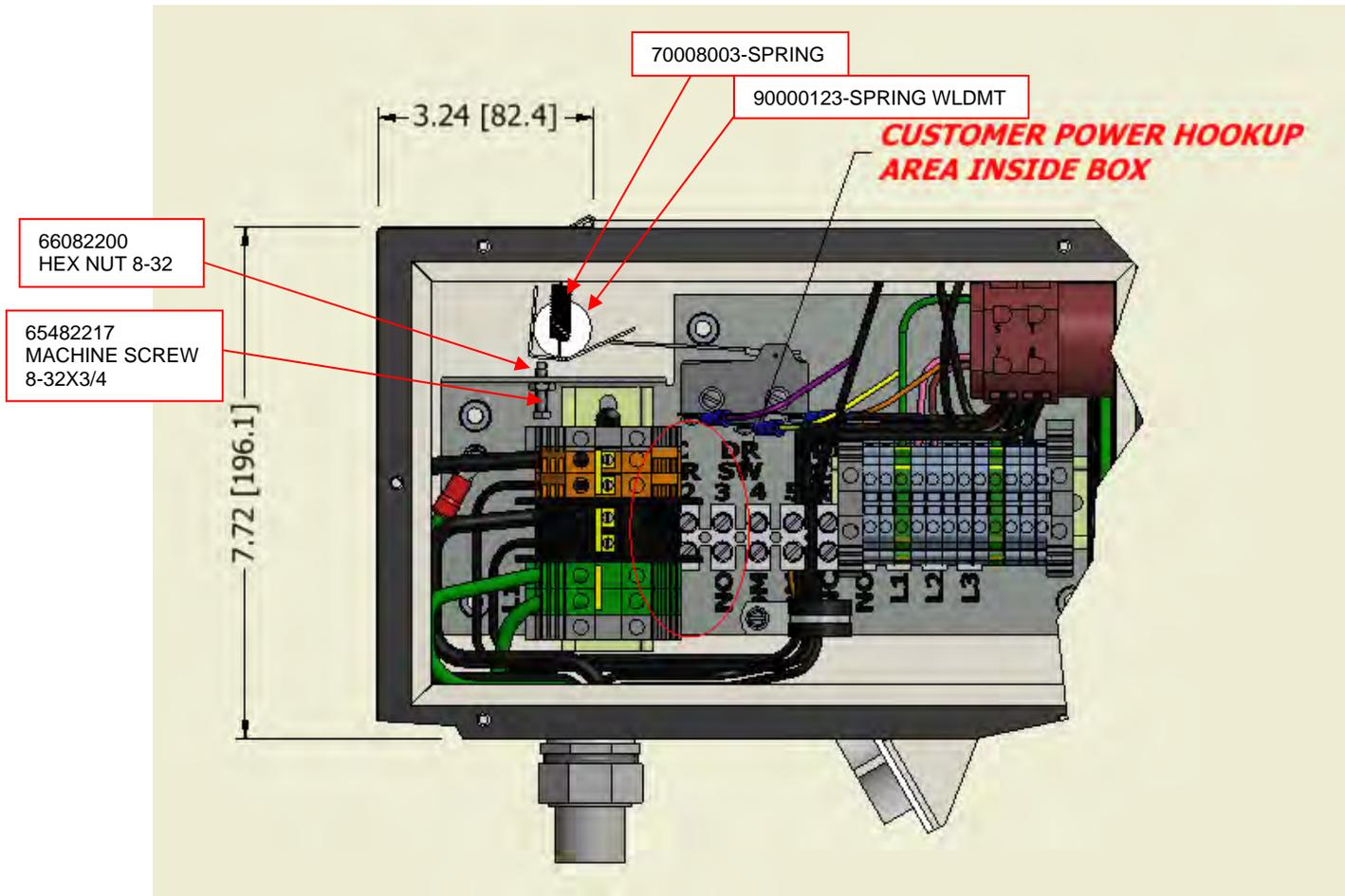
1. Back out the 65482217 adjusting screw and remove the 70008003 spring.
