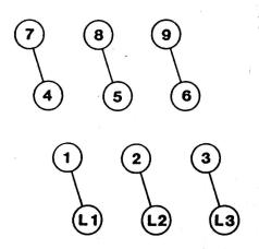
All 30 mill motors can be wired for 230 volt or 460 volt operation. See the specification sheets for 230 volt 3 phase motors for motor part numbers and other information.
