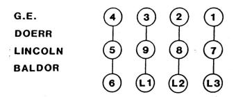
The mill motor may be operated with either CW or CCW rotation. To change rotation, reverse any two (2) of the black leads to the motor.
